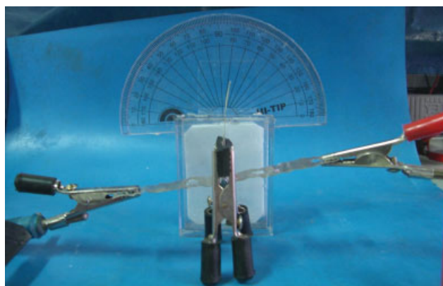
Figure 1 Experimental setup to measure degree of actuation. [Color figure can be viewed in the online issue, which is available at www.interscience.wiley.com .]
